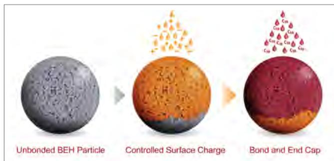
Charged Surface Hybrid (CSH) Technology improves selectivity and offers the highest possible performance for basic compounds in the acidic, low-ionic strength mobile phases commonly used in LC-MS laboratories.
