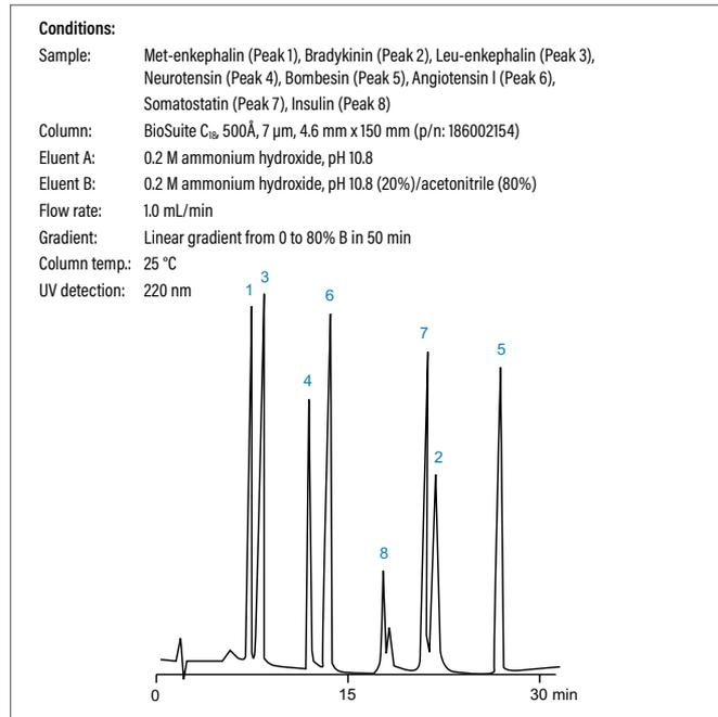
Use of "pH stable" methacrylate-based particles contained in Waters BioSuite pC<sub>18</sub> Reversed-Phase Columns allow scientists to change separation selectivity by using a pH not possible with 100% silica-based C<sub>18</sub> columns.
