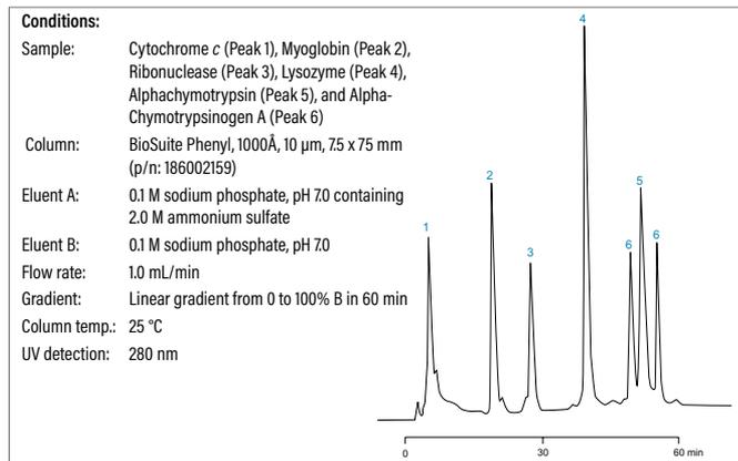
The BioSuite Phenyl, 1000Å HIC Columns have a lower ligand density compared to the BioSuite pPhenyl, 1000Å RPC Columns and are not recommended for reversed-phase separations.
