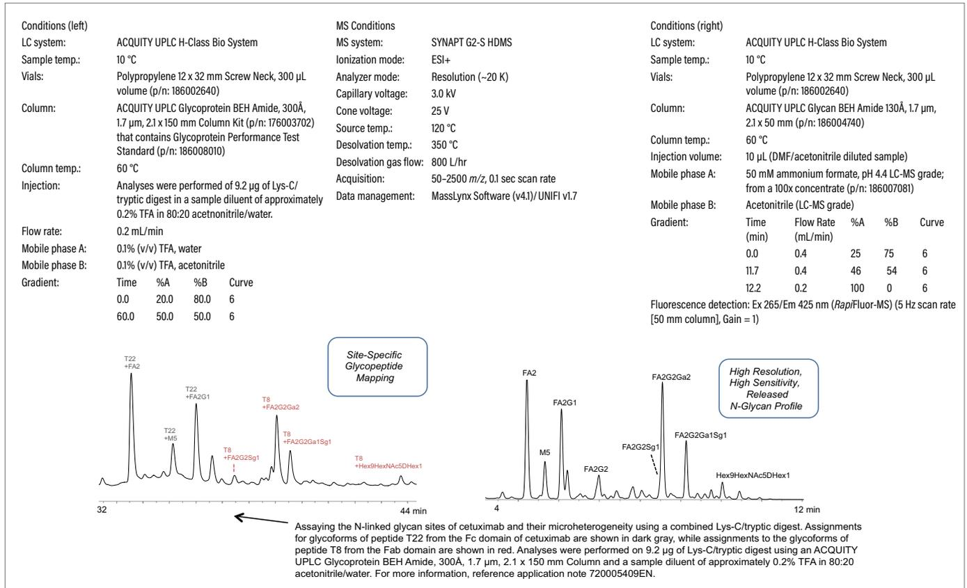
HILIC Profiling of cetuximab glycosylation. HILIC-fluorescence chromatograms of RapiFluor-MS labeled N-glycans from cetuximab obtained using an ACQUITY UPLC Glycan BEH Amide, 300Å, 1.7 µm, 2.1 x 50 mm Column. Mass spectral data supporting the assignments of the RapiFluor-MS labeled N-glycans are provided.
