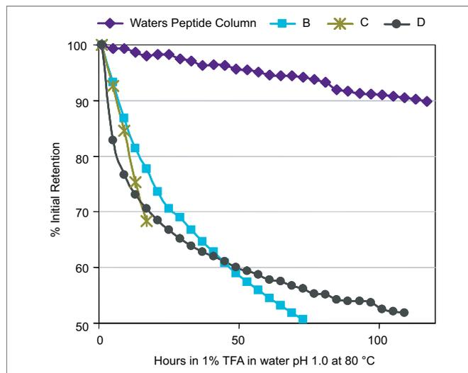
We tested several peptide columns to observe how they performed when injections were repeated, comparing them with the performance columns B, C, and D, made by other manufactures. (Retention was monitored to determine column lifetime.)
