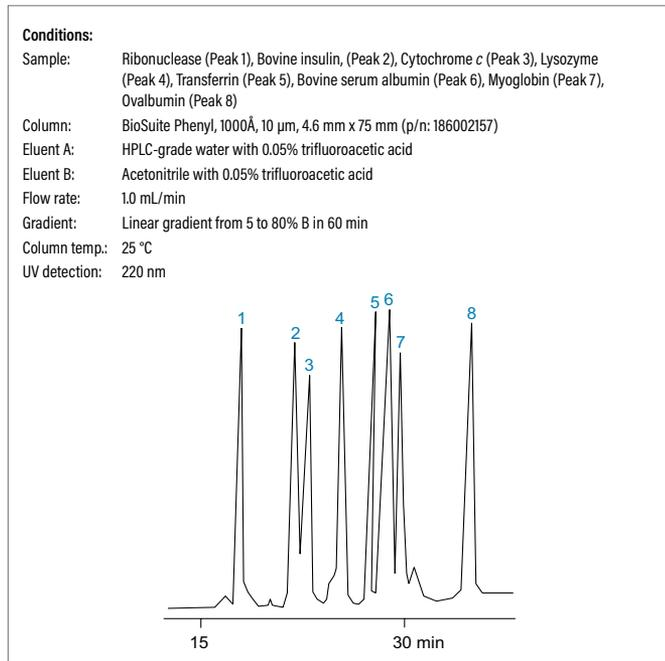
The BioSuite pPhenyl, 1000Å RPC Columns have a higher ligand density compared to the BioSuite Phenyl, 1000Å HIC Columns and are not recommended for hydrophobic-interaction separations.
