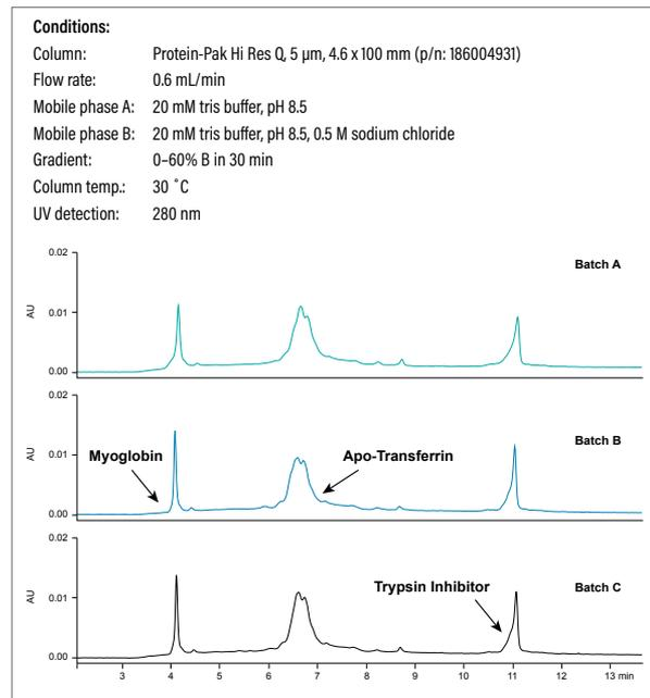
Each batch of Protein-Pak Hi Res SP, CM, and Q Column packing material is chromatography tested using a relevant protein standard mixture to help ensure consistent and predictable performance.
