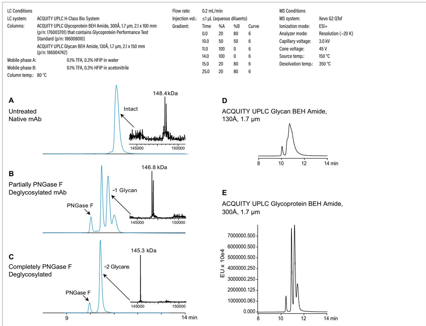
Glycoprotein BEH Amide, 300Å, 1.7 µm Column analyses of Waters mAb Mass Check Standard showing native (A), partially deglycosylated (B), and completely deglycosylated (C) samples. Also showing HILIC fluorescence profiles of partially deglycosylated Intact mAb Mass Check Standard using two ACQUITY UPLC Glycan BEH Amide, 130Å, 1.7 µm, 2.1 x 150 mm Columns in series (D) versus two ACQUITY UPLC Glycoprotein BEH Amide, 300Å, 1.7 µm, 2.1 x 150 mm Columns in series (E).
