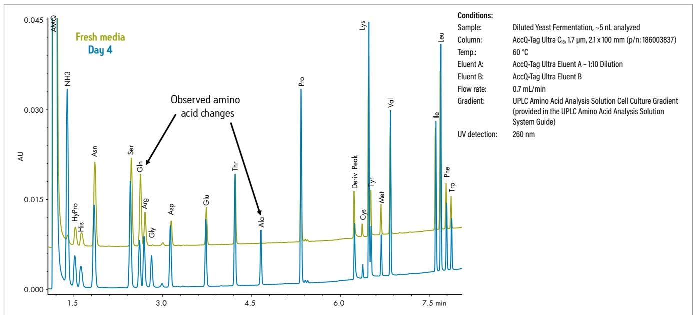
Amino acid levels in a growing cell culture change over a relatively short period shown here as a decrease in glutamine accompanied by an increase in alanine. The supplied methods were used without modification and no sample prep beyond dilution was required.
