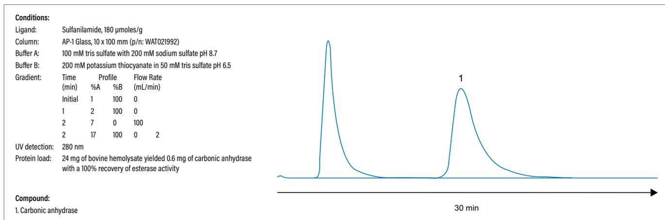
Waters Protein-Pak Affinity material can be successfully used to create an affinity resin as shown in the example of the affinity purification for the protein carbonic anhydrase.
