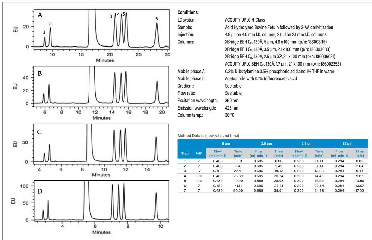
Geometric scaling of a monosaccharide separation on XBridge BEH C<sub>18</sub>, 130Å, (A) 5  $\mu$ m particle, (B) 3.5  $\mu$ m particle, (C) 2.5  $\mu$ m particle, and (D) 1.7  $\mu$ m particle noting higher throughput and improved component Rs via use of 1.7  $\mu$ m particle technology.
