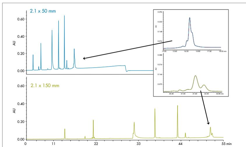
*Increasing the length of the column will increase the resolving power for a separation. This is shown with the separation of a protein mixture. The additional small peaks surrounding the Phosphorylase b can be seen more readily on the longer column, as seen in the inset, but it comes at the cost of a 3-fold increase in run time and ~40% loss of sensitivity. Depending on the application objective, this may be a useful parameter to improve resolution.*
