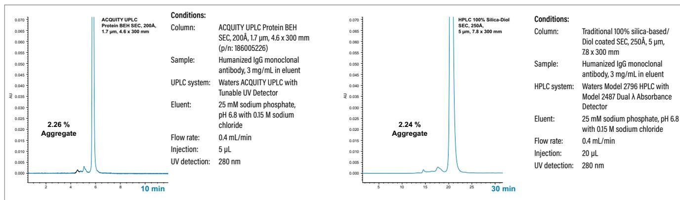
Compared to use of traditional HPLC-based SEC technology, Waters ACQUITY UPLC BEH SEC Technology delivers benefits of the comparable determination on mAb aggregate vs. monomer (i.e., less time, higher sample throughput).
