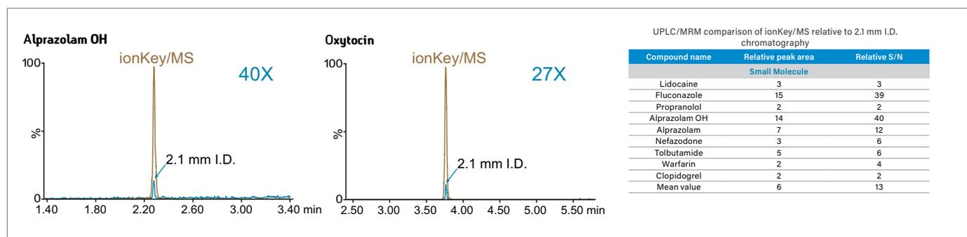
Sensitivity comparison between ionKey/MS and 2.1 mm I.D. chromatography; 1 µL injection of equal sample load on each.
