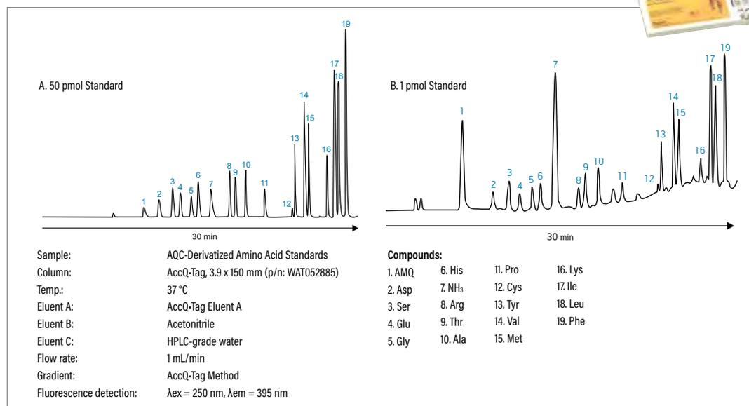
*Application of the AccQ-Tag Method to the analysis of hydrolysate amino acids is illustrated. The high purity reagents provided in the AccQ-Tag Chemistry Package enable high sensitivity analysis by minimizing background amino acid content. AMQ (6-Aminoquinoline).*
