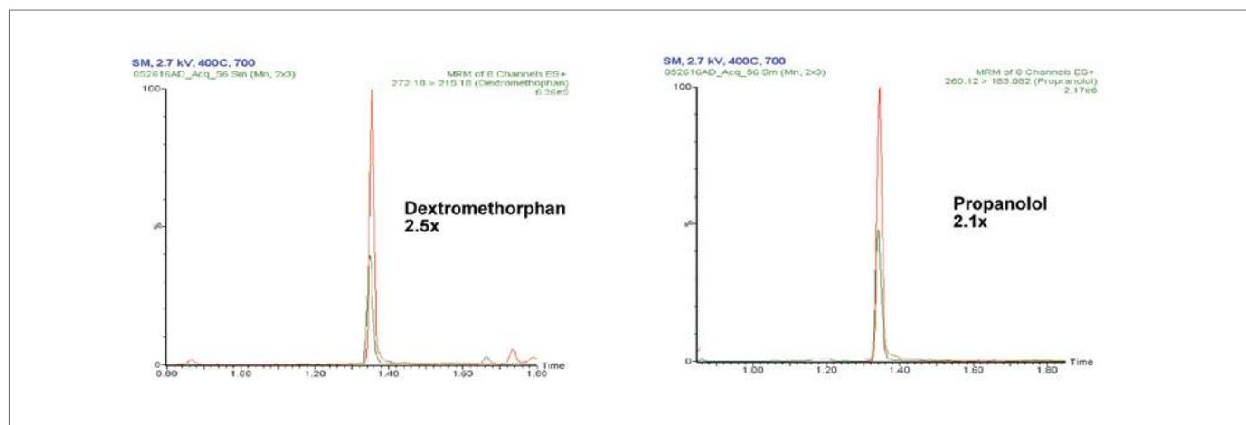
Sensitivity gains using (300 µm × 50 mm) iKey HT BEH C<sub>18</sub> Separation Device (red) compared to (2.1 mm × 50 mm) UPLC BEH C<sub>18</sub> Column (green) under identical injection volume and gradient conditions.
