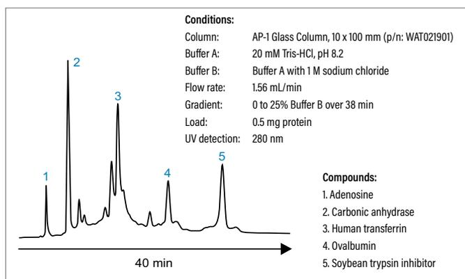
Waters Advanced Purification (AP) Glass Columns, containing Protein-Pak DEAE 15 µm particles, are well suited for the analysis and/or lab-scale purification of various protein mixtures.
