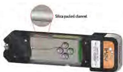
iKey Separation Device with Post Column Addition (PCA)
