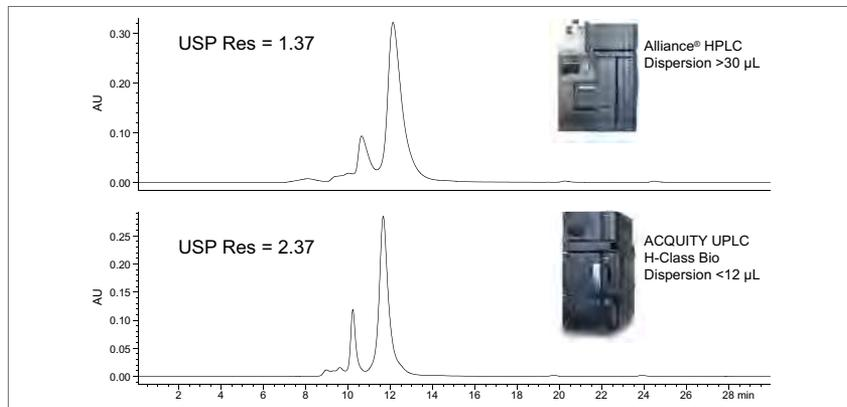
*The extra system volume of the traditional HPLC System (top) caused the column separated peaks to “partially remix” resulting in a USP resolution factor of 1.37 vs. the superior 2.37 value obtained when the separation was performed on an ACQUITY UPLC System. This slide shows how the LC system’s “band broadening” can adversely affect the quality of the mAb separation generated with the same XBridge® Protein BEH SEC, 200Å, 2.5 µm Column, SEC eluent, and sample.*
