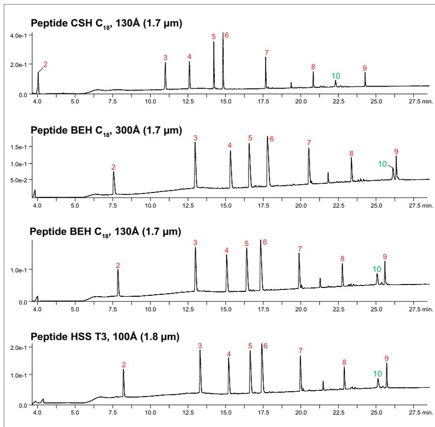
Peptides contained in Waters MassPREP Peptide Standard Mixture, p/n: [186002337](#), were separated on 2.1 × 150 mm columns containing Waters Peptide CSH C<sub>18</sub> 130Å (1.7 µm), Peptide BEH C<sub>18</sub> 300Å (1.7 µm), Peptide BEH C<sub>18</sub> 130Å (1.7 µm), or Peptide HSS T3 100Å (1.8 µm) UPLC-based particles on a Waters H-Class Bio System using a gradient of increasing acetonitrile concentration with 0.1% FA ion-pairing. Flow at 0.2 mL/min.
