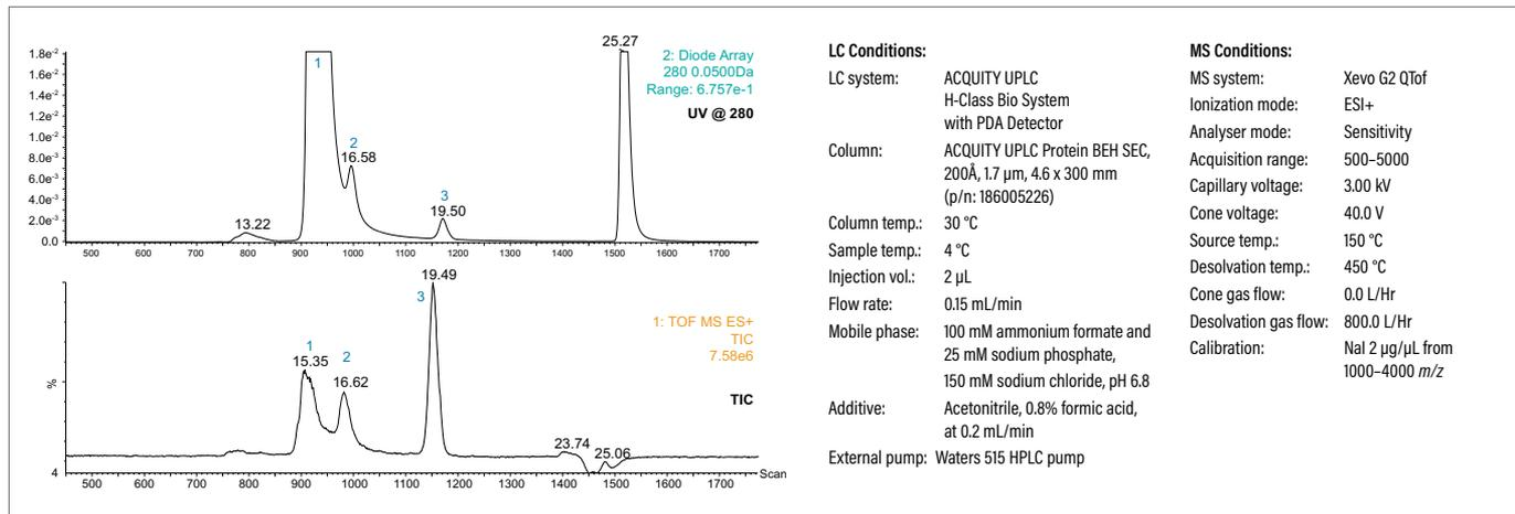
An intact biotherapeutic mAb, which was past expiry, was analyzed by using MS-friendly, non-denaturing conditions. In the UV chromatogram, not only are the mAb aggregate and monomer observed, but a low molecular weight (LMW) peak eluting after the intact mAb is partially resolved as well. In addition to these peaks, the UV chromatogram reveals two other LMW species.
