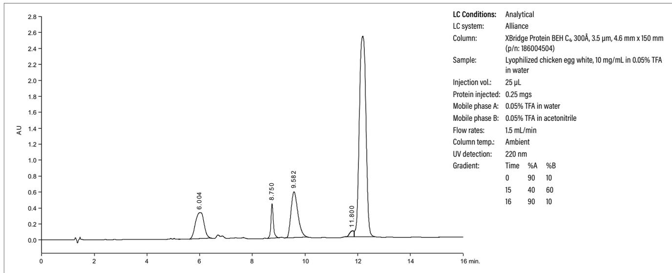
Analytical scale separation of 250 μg chicken egg white proteins on XBridge Protein BEH C<sub>4</sub>, 300Å, 3.5 μm, 4.6 x 150 mm Column.
