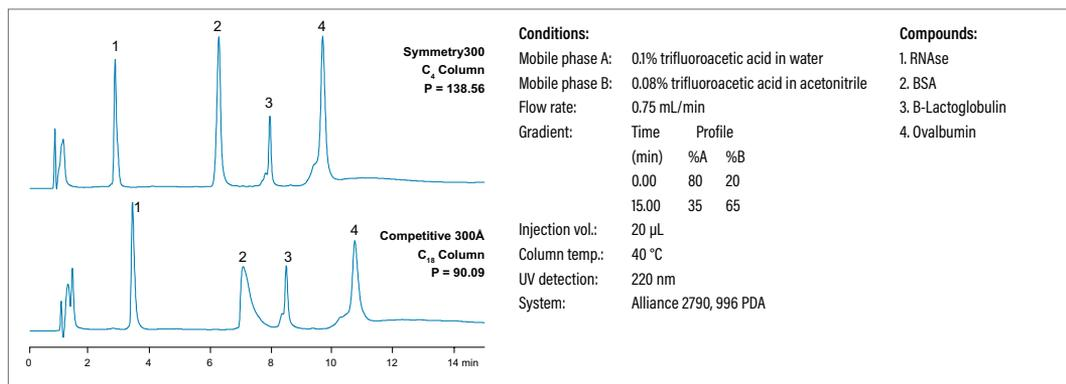
*Compared to many competitive 100% silica-based C<sub>18</sub> columns, Waters proprietary bonding and end-capping technologies help deliver improved peak shape with less undesired tailing.*
