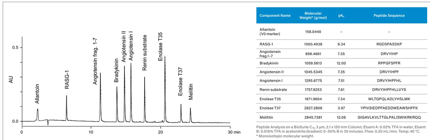
Waters offers a variety of carefully formulated and QC-tested peptide standards to help chromatographers confirm the performance of their column and LC system prior to analyses of potentially highly valued samples.
