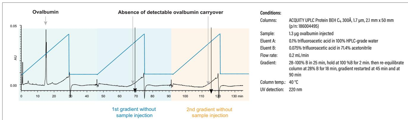
Column carryover was tested by running multiple gradients following a single injection. Protein peaks observed during the first gradient are not found in subsequent gradients.
