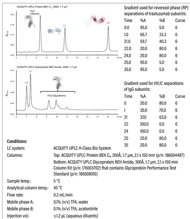
Trastuzumab subunit separations. (A) 1 µg of reduced, IdeS digested separated using an ACQUITY UPLC Protein BEH C<sub>4</sub>, 300Å, 1.7 µm Column (0.7 µL aqueous injection). (B) 1 µg of reduced, IdeS digested separated using an ACQUITY UPLC Glycoprotein BEH Amide, 300Å, 1.7 µm Column (0.7 µL aqueous injection).
