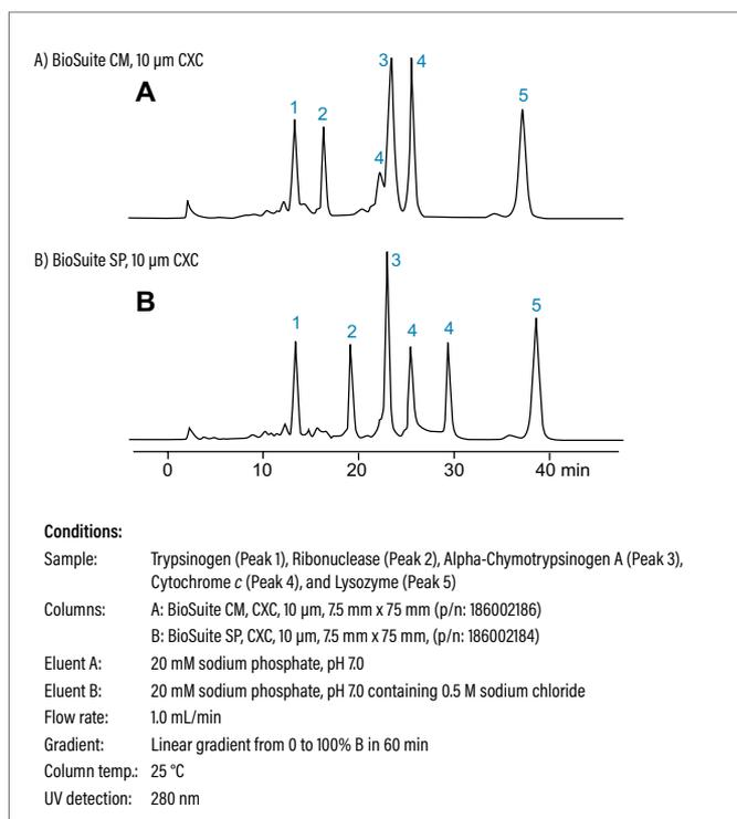
*BioSuite strong (SP) and weak (CM) cation-exchange columns deliver different separation selectivities useful when developing a method to adequately separate a complex biocompound mixture.*
