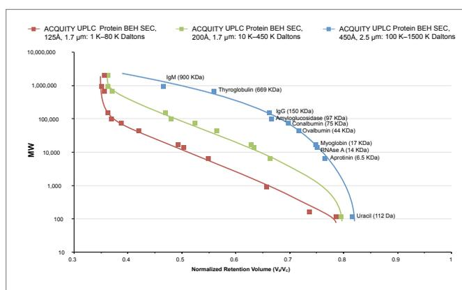
Size exclusion chromatography (SEC) separates compounds primarily based on their relative size in solution. Calibration curves on Waters HPLC-based, SEC Columns of different pore size, using defined protein and peptides of known molecular weight, help chromatographers select the most appropriate SEC column for their specific application.
