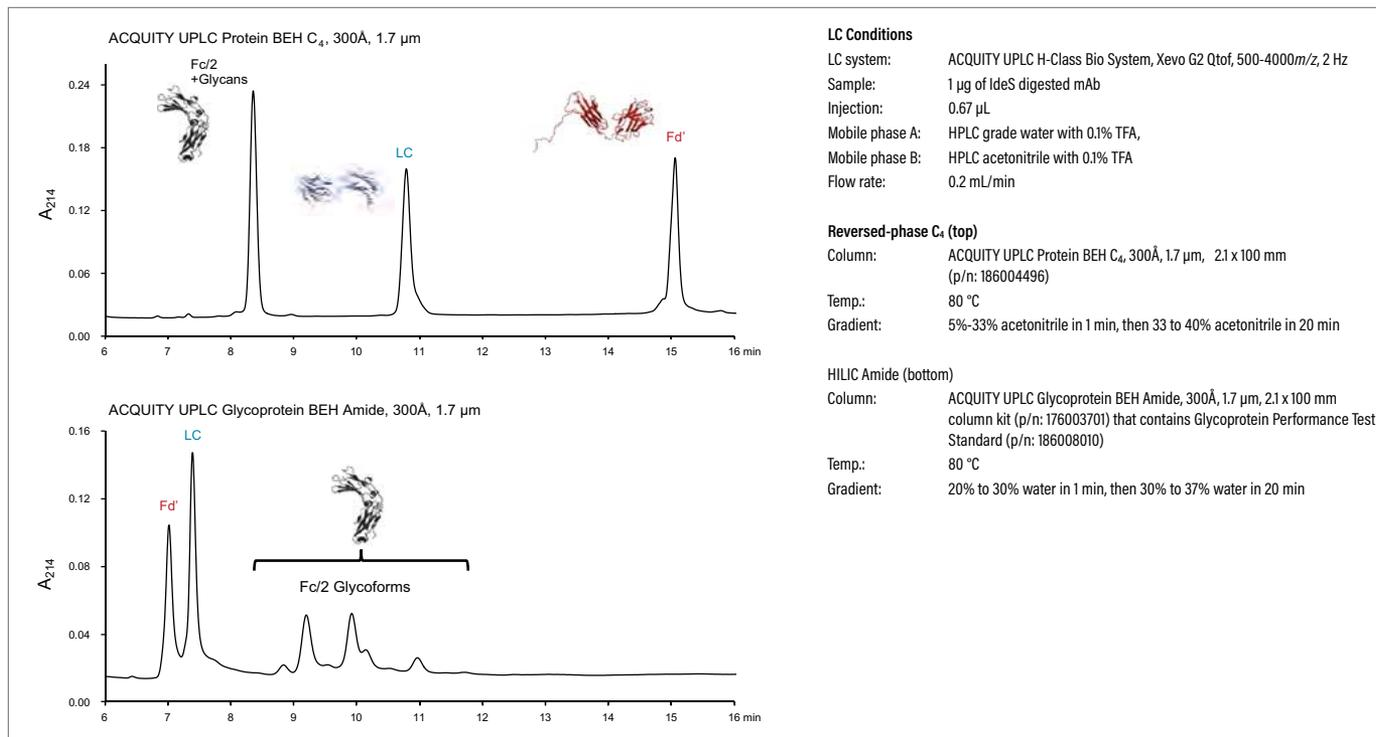
Trastuzumab subunit separations. Top: 1 µg of reduced, IdeS digested separated using an ACQUITY UPLC Protein BEH C<sub>4</sub>, 300Å, 1.7 µm Column (0.7 µL aqueous injection). Bottom: 1 µg of reduced, IdeS digested separated using an ACQUITY UPLC Glycoprotein BEH Amide, 300Å, 1.7 µm Column (0.7 µL aqueous injection).
