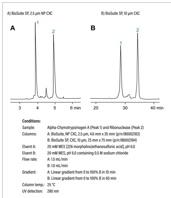
*Use of 2.5 µm, superficially-porous particles, contained in the BioSuite SP NP Columns, can deliver improved peptide component resolution and in less time (left figure) compared to the use of a BioSuite SP, CXC column that contains 10 µm, fully-porous particles (right figure).*
