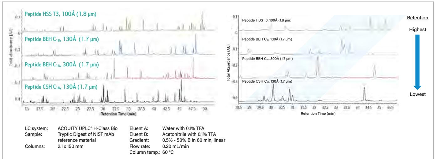
Waters UPLC (shown) and HPLC-based, Peptide Separation Columns deliver different peptide selectivities and high peak capacities for the separation of complex peptide mixtures. In addition, each batch of material is specifically QC tested and qualified with a tryptic digest of cytochrome c to help ensure column to column consistency when used in validated methods.
