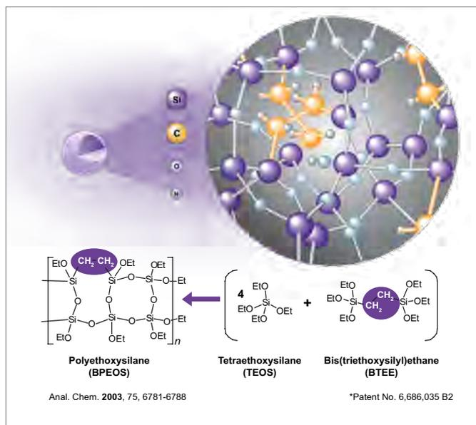
*Ethylene-Bridged Hybrid (BEH) Technology synthesis creates particles that ensure extreme column performance and long column lifetime under harsh operating conditions.*
