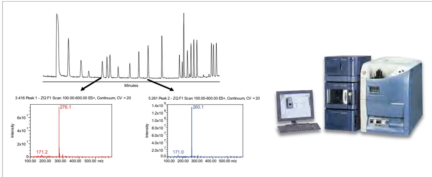
*The UPLC Amino Acid Analysis Application Solution is directly compatible with electrospray mass spectrometry.*
