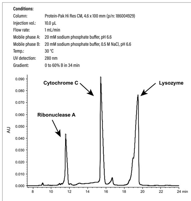
Waters offers a variety of carefully formulated and QC tested anion-exchange and cation-exchange protein standards to help chromatographers confirm adequate performance of their IEX column and LC system prior to the analyses of potentially highly valued samples.
