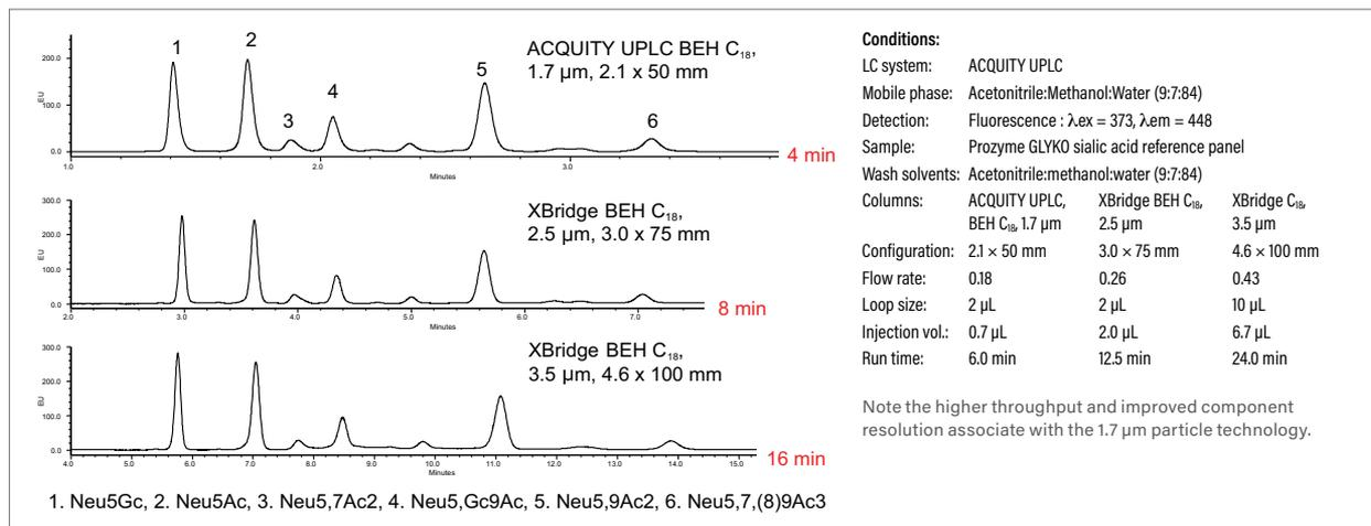
Geometric scaling of DMB-labeled sialic acid standards on XBridge BEH C<sub>18</sub>, 130Å, 3.5  $\mu$ m particle (bottom), 2.5  $\mu$ m particle (middle), and ACQUITY UPLC BEH C<sub>18</sub>, 130Å, 1.7  $\mu$ m particle (top).
