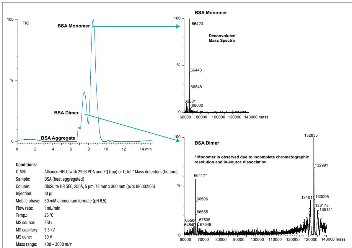
SEC is an effective technique to separate and quantitate higher molecular weight protein aggregates from lower molecular weight monomers using optical detection. Use of MS-compatible SEC eluents provides an additional dimension of useful data by providing real time mass data of the separated protein components.
