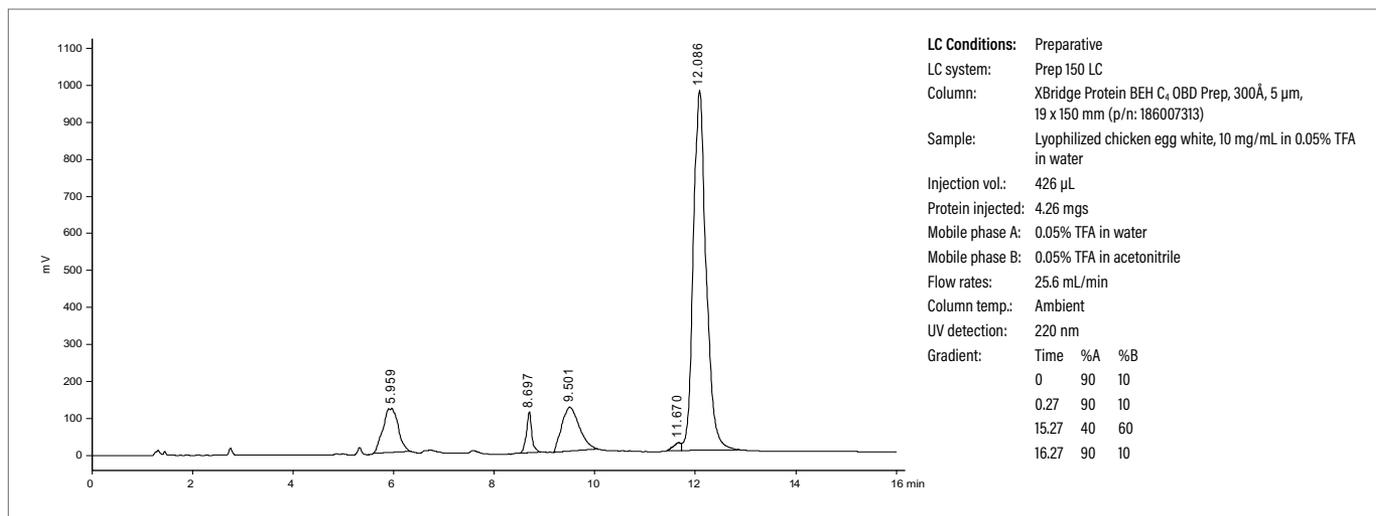
Effective method development and scaling of the 250 μm analytical scale separation to the preparative BEH C<sub>4</sub>, 300Å, 5 μm, 19 x 150 mm column results in chromatography showing an almost identical separation pattern.
