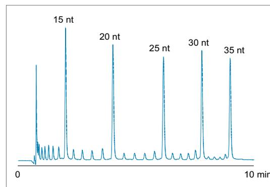
Waters ACQUITY UPLC analysis of MassPREP Oligonucleotide Standard on an ACQUITY UPLC Oligonucleotide C<sub>18</sub>, 1.7 μm Column. The main components are labeled. Small peaks eluting between labeled oligonucleotides are N-1, N-2, etc. failure sequences generated during the oligonucleotide syntheses. The ACQUITY UPLC System is equipped with 50 μL standard mixer and PDA Detector (260 nm).
