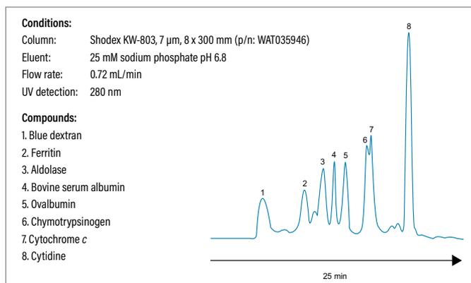
This gel-filtration separation of protein standards demonstrates the ability to separate proteins in a wide range of molecular weights in minutes for high sensitivity analysis or protein isolation up to the milligram scale.
