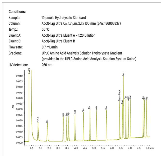
Separation of standard amino acids using the UPLC Amino Acid Analysis Solution Hydrolysate Method.
