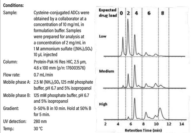
Monitoring drug load variability. Three batches of cysteine-linked ADCs were synthesized, each with a different level of drug conjugation (low, medium, high) and separated using hydrophobic interaction chromatography. The drug load distribution shifted from low to high corresponding to an increase in the load of the hydrophobic drug.
