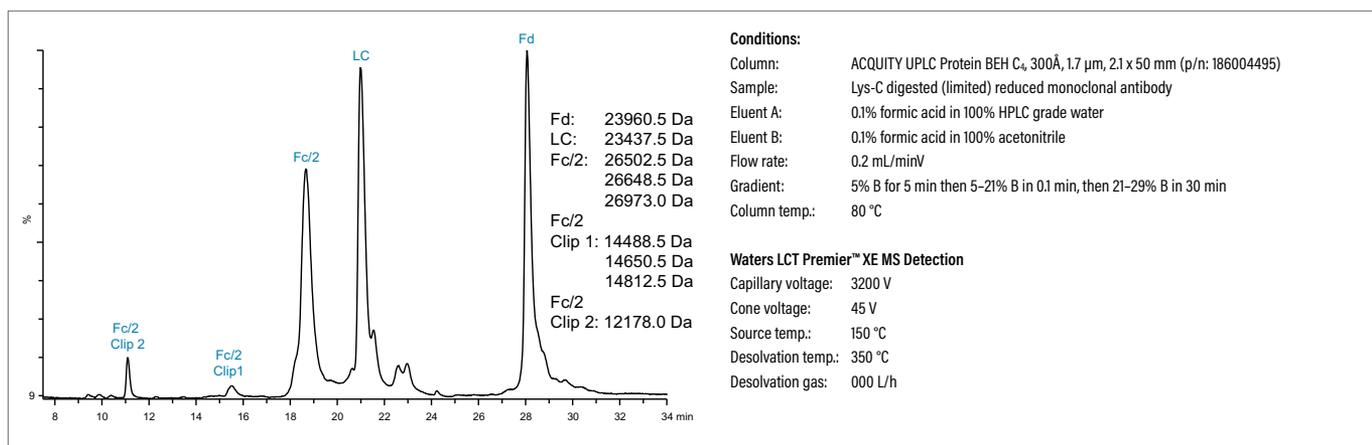
The large fragments obtained through LysC digestion of a monoclonal antibody can be separated on the ACQUITY UPLC Protein BEH C<sub>4</sub>, 300Å Column coupled directly to ESI/Tof MS for identification of the individual peptide products.
