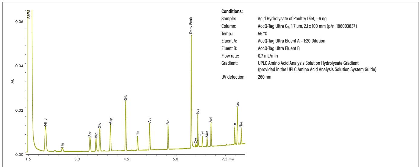
The 75 replicate analyses of a poultry diet mixed feed gives reproducible measurements of the weight percentage of the growth-limiting amino acids, typically 1% or better. The high sensitivity of the method ensures that only a very small aliquot of sample is required, thereby minimizing interferences.
