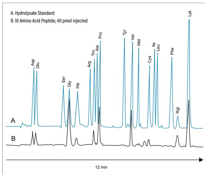
This 12-minute analysis using Waters Pico-Tag Amino Acid Analysis Method provides identification and accurate quantitation of the amino acid composition.
