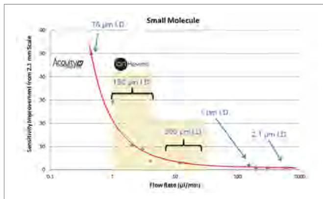
Sensitivity enhancement for a series of small molecules relative to a 2.1 mm I.D. separation performed on an ACQUITY UPLC System. The volume and concentration of sample injected on each column format was identical.
