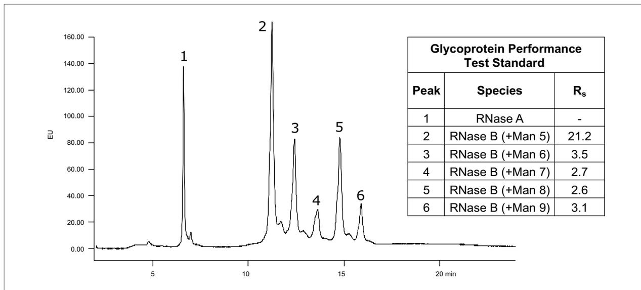
Separation of the Glycoprotein Performance Test Standard (RNase A + RNase B glycoforms) using an ACQUITY UPLC Glycoprotein BEH Amide, 300Å, 1.7 µm, 2.1 x 150 mm Column. Fluorescence detection at Ex 280 nm and Em 320 nm and a column temperature of 45 °C were employed in this example.
