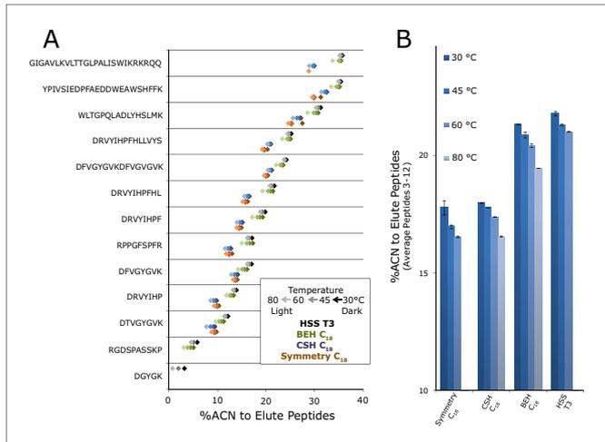
Peptide retention comparison of different stationary phases, including Symmetry Silica (the lower retention of Symmetry is used in trap-elute separations).
