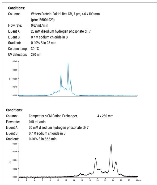
Cation-exchange chromatography is a useful tool for the characterization and quantitation of mAb or recombinant protein variants. Use of Waters Protein-Pak Hi Res CM Column on an ACQUITY UPLC System increases sample throughput while maintaining resolution between intended product and undesired variants.
