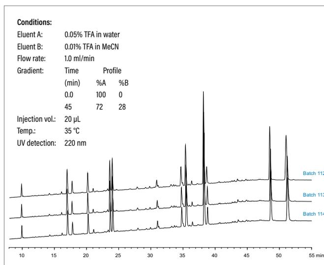
Waters BioSuite C<sub>18</sub> PA-A and PA-B Columns are QC tested with tryptic digest of cytochrome c (p/n: 186006371) to help ensure batch-to-batch and column-to-column performance consistency.
