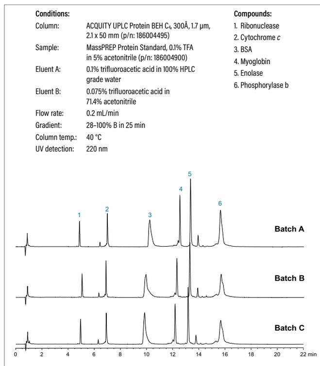
Waters MassPrep Protein Standard Mixture is used to critically QC test the ACQUITY UPLC Protein BEH C<sub>4</sub>, 300Å Columns to help ensure consistent batch-to-batch and column-to-column performance.
