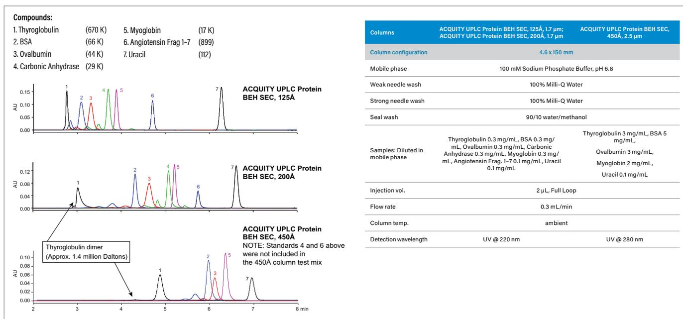
Waters offers a family of BEH-based, diol-coated SEC columns of different pore size to satisfactorily address the molecular weight range of analytes to be separated.
