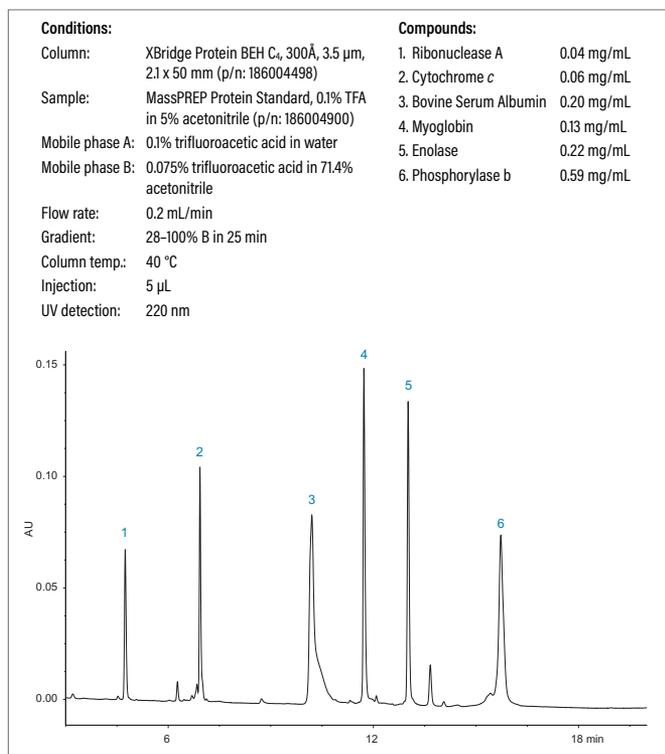
Protein BEH C<sub>4</sub>, 300Å Columns can be used with proteins that have a wide range of properties. This protein mix was chosen to represent a range of isoelectric points, molecular weights, and hydrophobicities.
