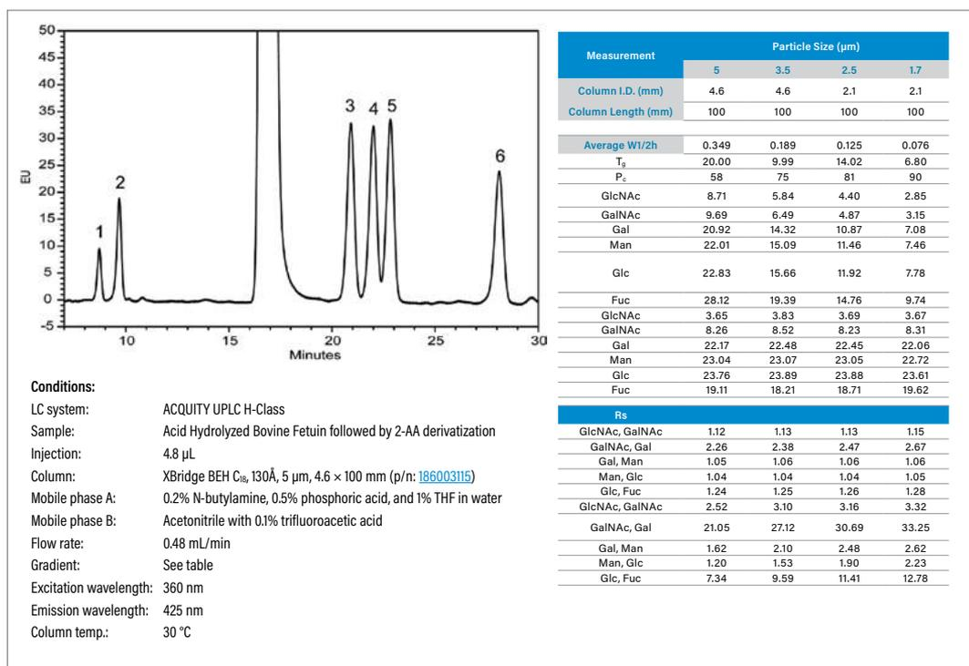
*HPLC analysis of monosaccharides. A separation performed with a Waters XBridge BEH C<sub>18</sub>, 130Å, 5 µm Column as detailed in Waters Applications Note: 720005255EN. Monosaccharides are identified as follows: (1) N-acetylglucosamine (GlcNAc), (2) N-acetylgalactosamine (GalNAc), (3) Galactose (Gal), (4) Mannose (Man), (5) Glucose (Glc), and (6) Fucose (Fuc).*
