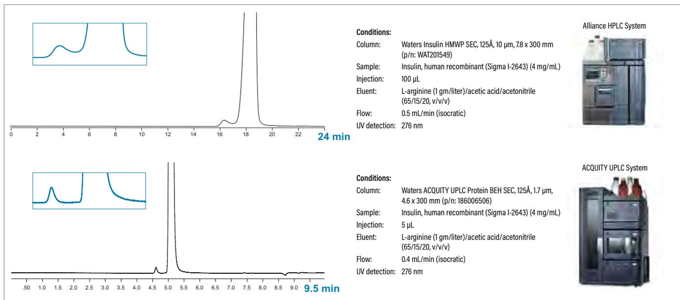
Compared to use of traditional HPLC-based SEC technology for the analysis of earlier eluting insulin aggregates from desired monomer species, Waters ACQUITY UPLC BEH SEC Technology delivers benefits of improved component resolution and in less time.
