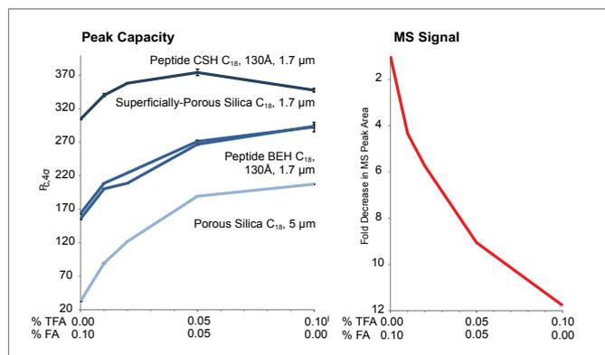
Effect of trifluoroacetic acid on peak capacity and MS signal. (A) Peak capacity as a function of acid modifier. Values were derived from two replicates. (B) Fold decrease in MS peak area as a function of acid modifier. Waters MassPREP Peptide Standard Mixture (p/n: 186002337) was used in study.
