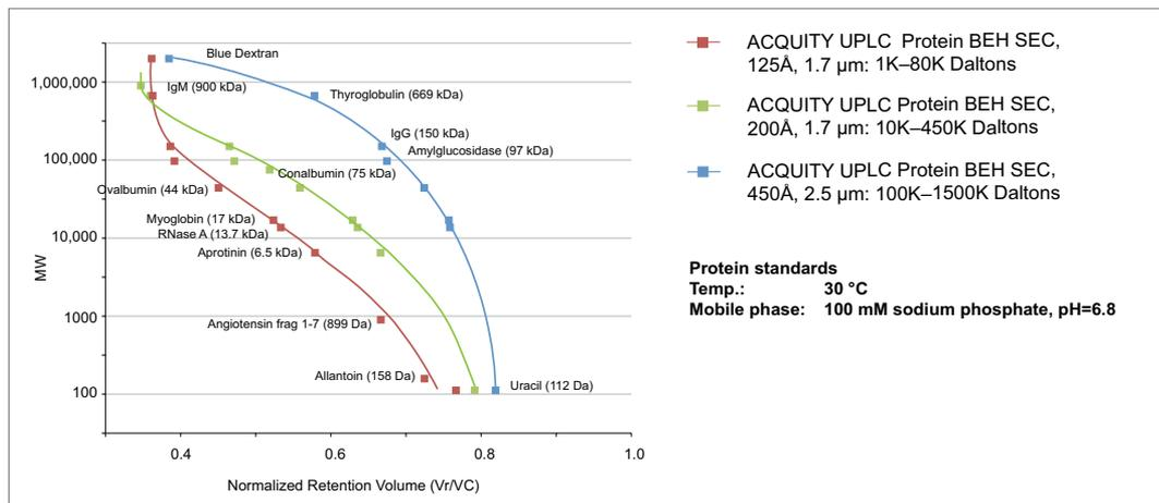
*Size exclusion chromatography (SEC) separates compounds primarily based on their relative size in solution. Calibration curves on UPLC-based SEC columns of different pore size, using defined protein and peptides of known molecular weight, help chromatographers select the most appropriate SEC column for their specific application.*
