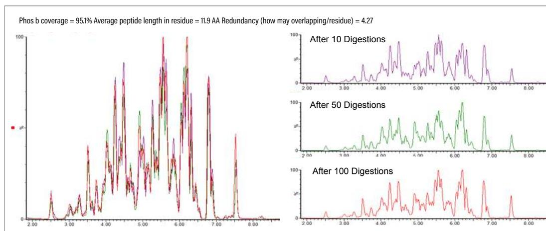
Reproducible online pepsin digestions of phosphorylase b. A total of 130 digestions were performed using an Enzymate Pepsin Column. The 10<sup>th</sup>, 50<sup>th</sup> and 100<sup>th</sup> digestions are shown. The sequence coverage is shown on the right.
