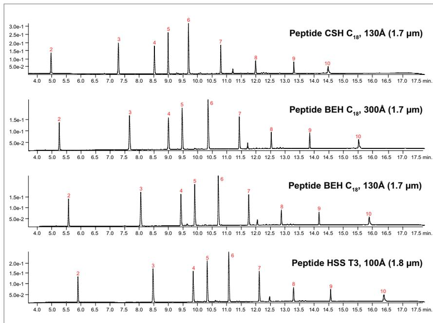
Peptides contained in Waters MassPREP Peptide Standard Mixture, p/n: [186002337](#), were separated on 2.1 × 150 mm columns containing Waters Peptide CSH C<sub>18</sub> 130Å (1.7 µm), Peptide BEH C<sub>18</sub> 300Å (1.7 µm), Peptide BEH C<sub>18</sub> 130Å (1.7 µm), or Peptide HSS T3 100Å (1.8 µm) UPLC-based particles on a Waters H-Class Bio System using a gradient of increasing acetonitrile concentration with 0.1% TFA ion-pairing. Flow at 0.4 mL/min.
