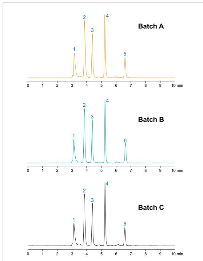
Waters BEH Protein Standards (125Å, 200Å, and 450Å formulated mixtures) are used to critically QC test our Protein BEH SEC columns to help ensure consistent batch-to-batch and column-to-column performance.
