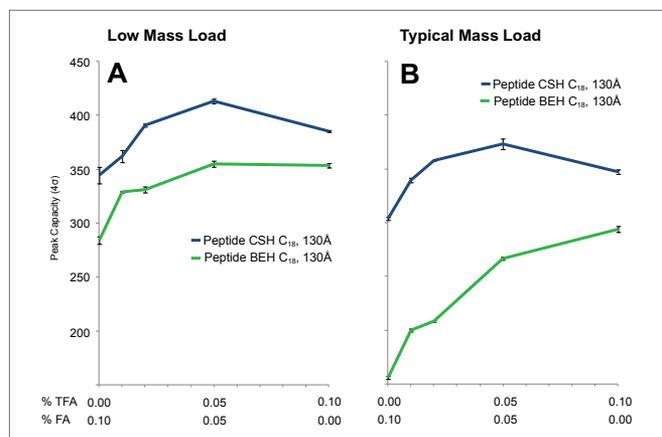
Effect of column mass load on separated peptide peak capacity in formic acid, trifluoroacetic acid, and eluent blends of formic acid and trifluoroacetic acid. (A) approximate sample load of 0.06 μg peptide mixture. (B) approx. 0.6 μg peptide mixture. Values were derived from two replicates. Waters MassPREP Peptide Standard Mixture (p/n: 186002337) was used in the study.
