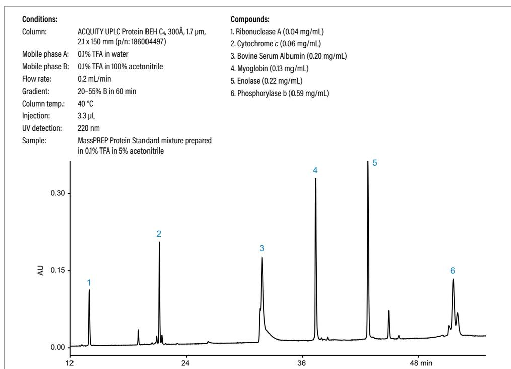
*Use of Waters carefully formulated and QC tested MassPREP Protein Standard Mixture can help chromatographers confirm adequate performance of their reversed-phase column and LC system prior to the analyses of potentially highly valued samples.*
