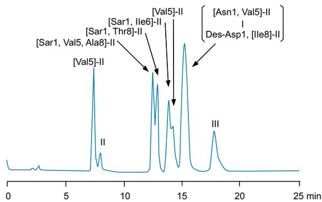
*Waters BioSuite SP-PEEK Cation-Exchange Column is well suited for the HPLC or UHPLC analyses of a complex peptide mixture using a gradient of increasing salt concentration.*
