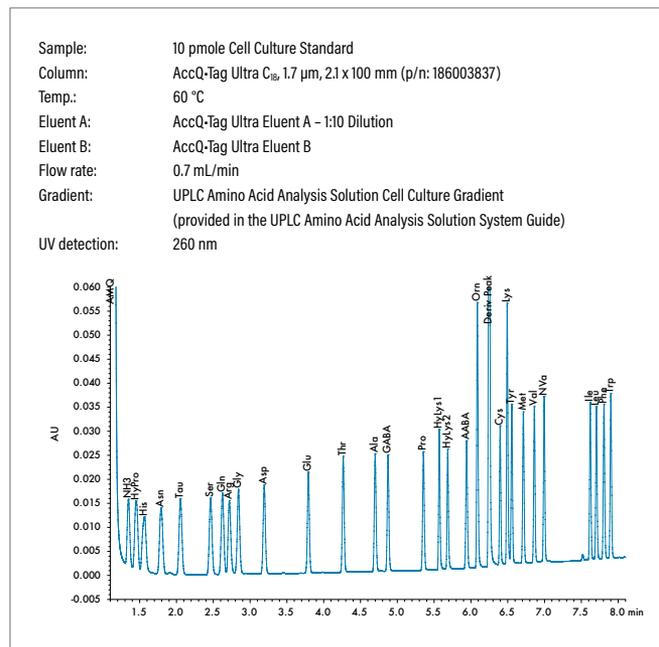
Separation of the larger set of standard amino acids using the UPLC Amino Acid Analysis Solution Cell Culture Method. No modification of the mobile phase pH or composition is required.
