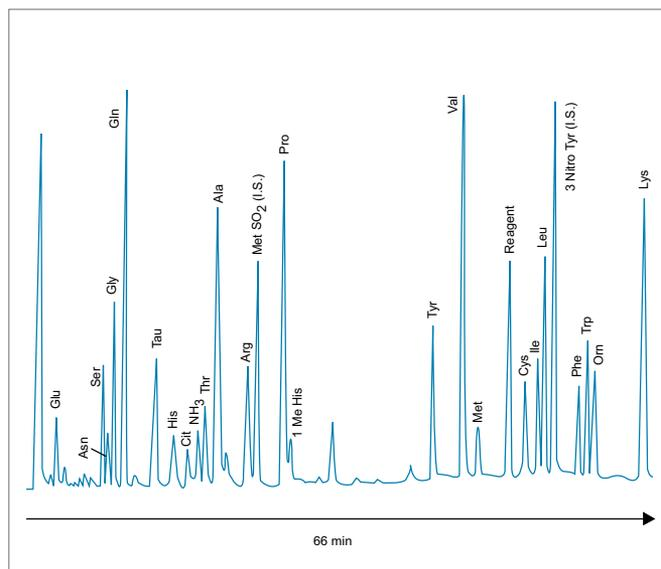
Reproducible and reliable plasma amino acid profiles are obtained in 66 minutes using Waters Pico-Tag Method. In this analysis, 100  $\mu\text{L}$  plasma was diluted with an internal standard, deproteinized by centrifugal ultrafiltration, and derivatized. The methionine sulfone (internal standard) peak represents 25 picomoles. Courtesy of A.S. Feste, R.W. Drummond, and S.J. Dudrich, Nutritional Support Service, St. Luke Episcopal Hospital, Houston, Texas.
