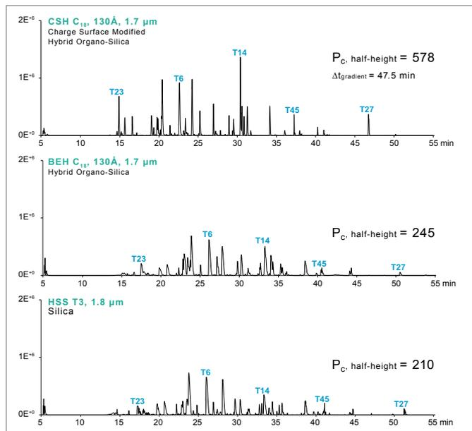
Comparison of a base peak ion chromatogram of MassPREP Enolase Digestion Standard, 1  $\mu\text{g}$ , direct injection on a 75  $\mu\text{m}$  (I.D.) column.
