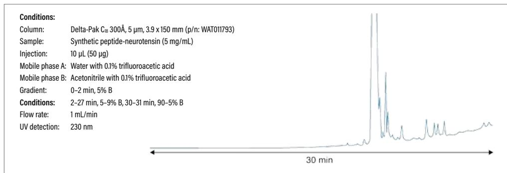
Waters Delta-Pak C<sub>18</sub>, 300Å Columns (available in 5 µm and 15 µm particle sizes) are well suited for the analysis and lab-scale isolation of synthetic peptide mixtures.
