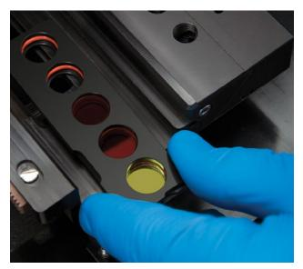
Figure 2. Integrated Filter Slides for GloMax<sup>®</sup> Discover and Explorer.
