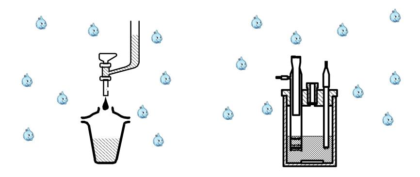
At 20°C and a relative air humidity of 60%, 1 L of air contains 12 mg of water
