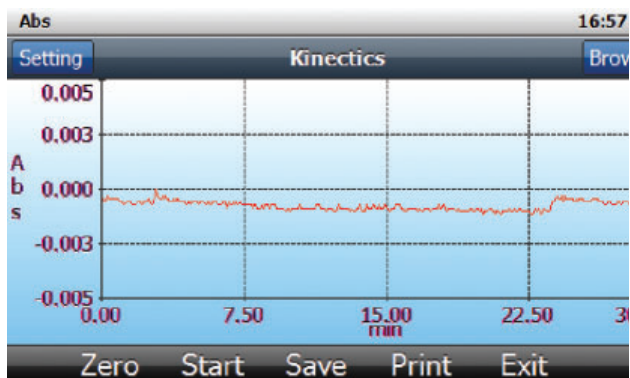
The Kinetic workspace enables the measurement of Absorbance or Transmission as a function of time. Use the zoom and peak pick features to obtain a better view of the Kinetic curve. Measurement data can be saved and recalled at any time.
